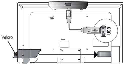
\* Attach the RF Dongle aligning with the upper left corner bracket.
